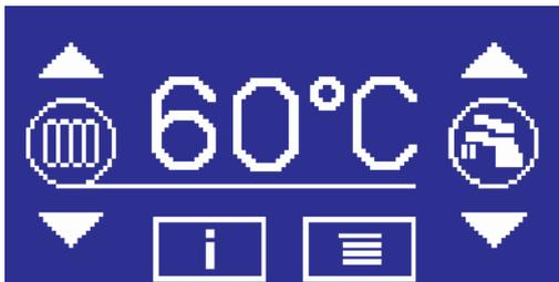
**DISPLAY OF HEATING WATER TEMPERATURE**
