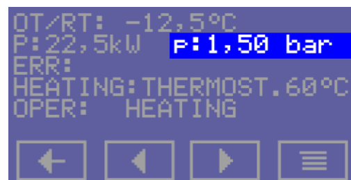
p: PRESSURE IN THE HEATING SYSTEM
