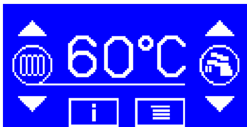
HEATING OF DHW ON
